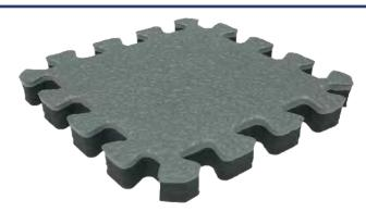
Active-Flex is an interlocking, multi-layer cushioned activity tile. The 4mm surface wear layer is a specially formulated rubber and synthetic mix which provides a non-porous surface for easy and hygienic cleaning. The surface also has a textured anti-slip finish.
