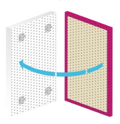
After waiting for the adhesive to slightly dry (2-5 minutes at 23°C) carefully align the panel to the marked area and push gently - allowing the clip spikes to bite into the panel. Once confident with the panel positioning, press firmly over the entirety of the surface and ensure maximum contact has been made with the wall.
