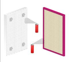
Spray the contact adhesive vertically onto the panels reverse surface and horizontally onto the desired installation area, including the impaling clips. Ensure that 100% of the surface area on both surfaces is covered with the adhesive.
