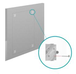
Lightly trace the panel edges onto the desired installation area then suitably and securely fix the appropriate number of impaling clips using screws.
